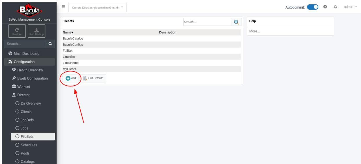
Here, we will start by creating a FileSet which will be used to backup one VMware VM managed by a vCenter server. We will use the 'vcenter-65' vCenter server which was configured in the “BWeb VMware Center” section of this document.
