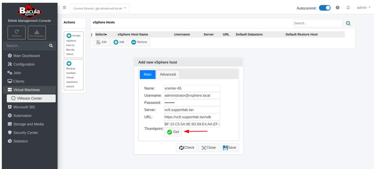
To get the “Thumbprint”, just click on the “Get” icon next to the Thumbprint field. Be sure that the “Server” IP address (or FQDN) is correct. It is important to verify this Thumbprint information now to prevent future issues or potential miscommunications with the wrong vSphere server.
