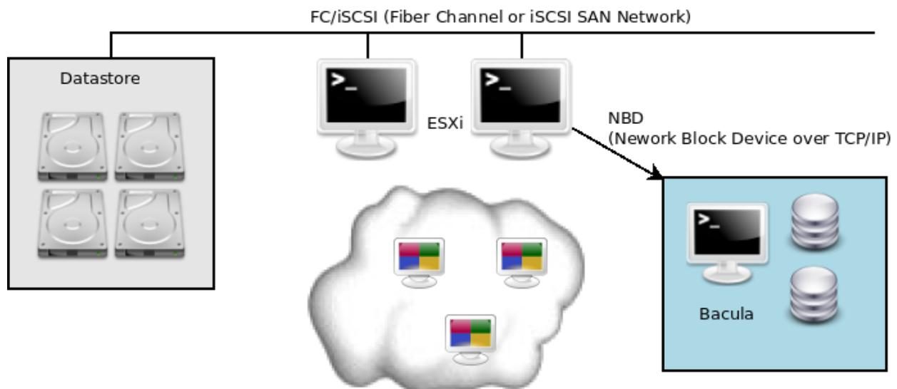
Fig. 1: Backup through TCP Network using NBD (Network Block Device)
