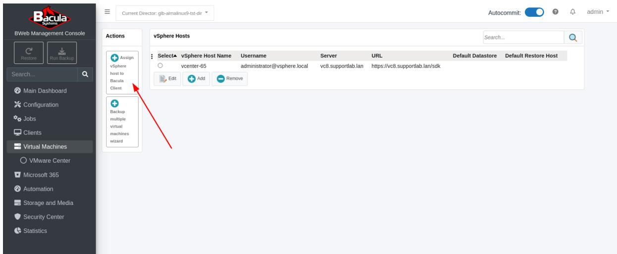
Next, we need to assign this vSphere (vCenter) host which we named “vcenter-65” to a Bacula FD with the vSphere plugin installed. To do this, click the “Assign vSphere host to Bacula Client” button in the upper left corner.
