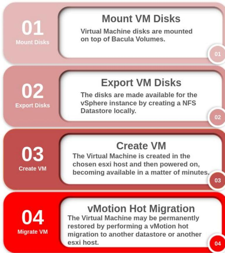
Any changes made to the VM disks are virtual and temporary. This means that the disks remain in a read-only state. The users may write to the VM disks without the fear of corrupting their backups. Once the Virtual Machine is started, it is then possible via VMotion to migrate the temporary Virtual Machine to a production datastore.
