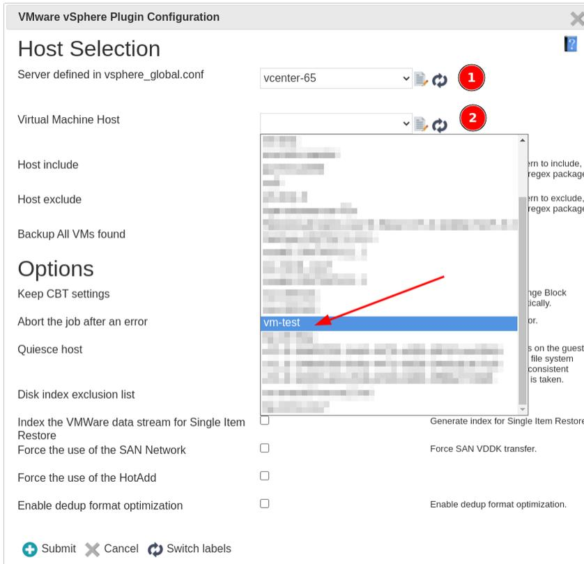
Since we are configuring a new FileSet and Job to backup one specific VM managed by this vCenter server, we will not use the “Host Include” and “Host Exclude” fields. These fields can be used to backup or exclude VMs based on wildcards like: `debian9-*` or `www-*`.
