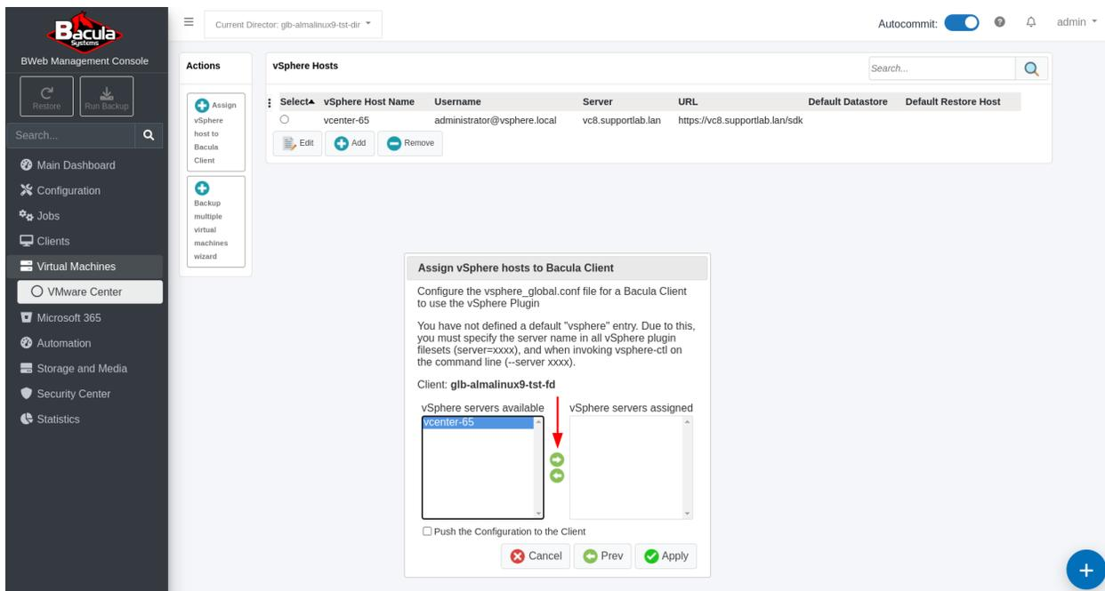
The “vcenter-65” vSphere host will be added to the “vSphere servers assigned” box on the right.
